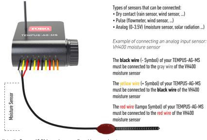
Note: the Tempus AG S1 has only one configurable sensor input.
